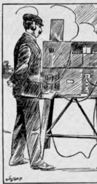
LODGE-MUIRHEAD PORTABLE WIRELESS TELEGRAPH PLANT. The Current is Generated by a Small Continuous-Current Motor Driven From a Stationary Bicycle.
